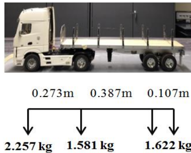
Figure 5-6: Model Bridge instrumented section for BWIM
