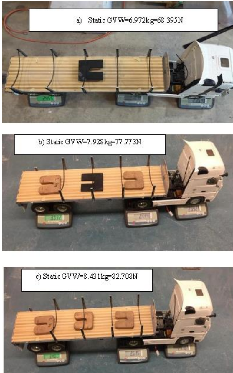
Figure 5-25 a, b, c: Static weight increments of model truck before each set of run
