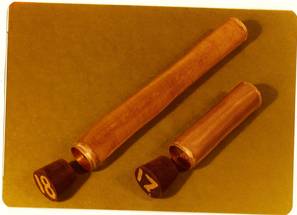
Figure 3.9 Wire Mesh Containers Used for Thermal Disinfestation Tests
