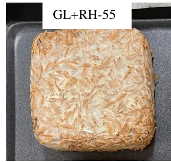
Figure 4.3 Comparison of appearance between compacted samples and uncompact samples. The number 40 on the picture's label represents uncompact samples, and 55 represents compacted samples.
