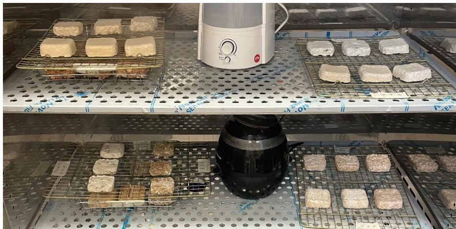
Figure 3.5 Moisture exposure testing
