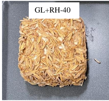
Figure 4.3 Comparison of appearance between compacted samples and uncompact samples. The number 40 on the picture's label represents uncompact samples, and 55 represents compacted samples.
