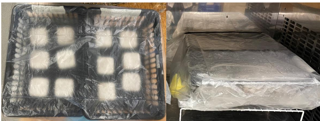
Figure 3.4 Demolded samples in the sealed baskets and cultivated in the incubator
