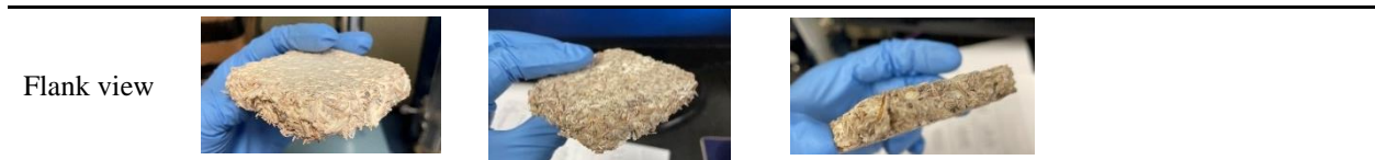
Figure 3.111 Top view and flank view of samples after compressive testing.
