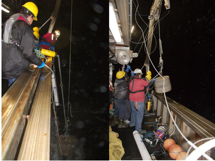
Figure 2.7. Example pictures of anchor-last deployment during SIMEP 2019 cruise.
