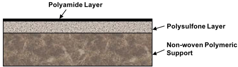
Figure 1. Cross-sectional view of three layered TFC membrane
