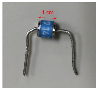
Fig. 4.2: The GDT Littelfuse 2027 series.
