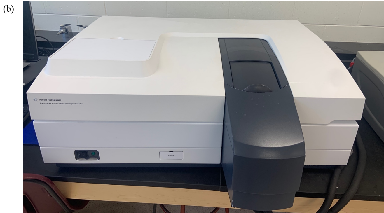
Figure 4. (a) schematic diagram of the basic components of a double-beam UV-Vis spectrophotometer. (b) Agilent Cary 5000 UV-Vis-NIR spectrophotometer.
