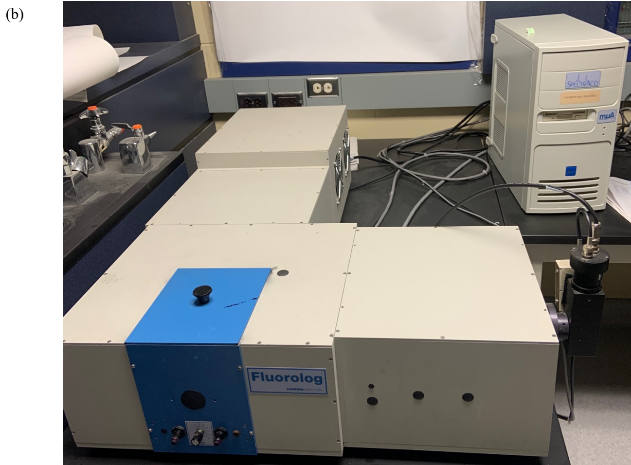
Figure 3. (a) schematic diagram of the typical constituents of a spectrofluorometer. (b) Fluorolog-3 Horiba Jobin Yvon Spectrofluorometer.
