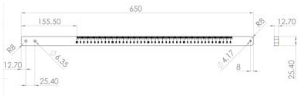
Figure 6: Measuring Block Assembly
