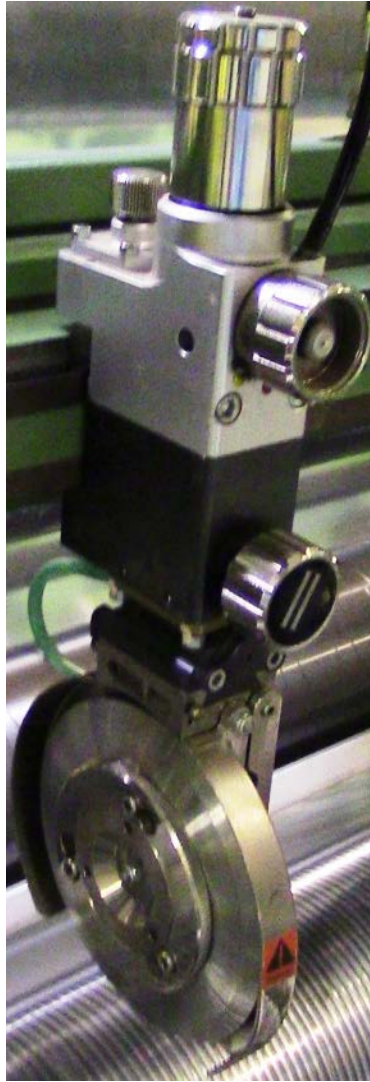
Figure A 10: Male slitter blade assembly [2]
