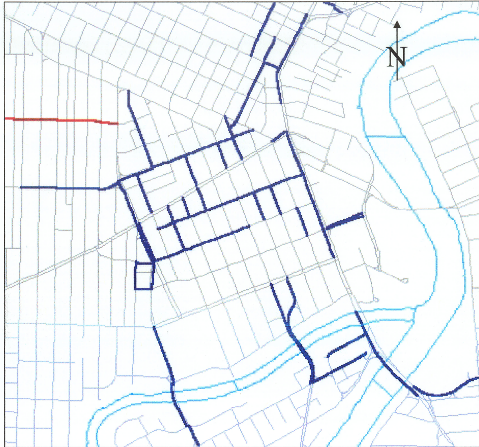
Figure 5.12: Enlargement of downtown Winnipeg showing anomalies between the manual and automated rating systems. Blue segments have IRI > 3.00 m/km and a general condition of good.
