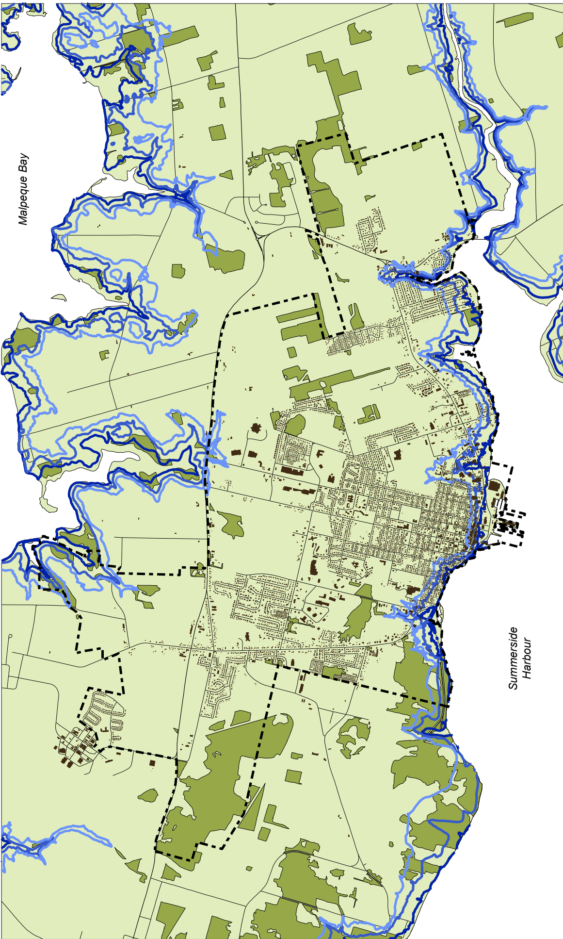
TOPOGRAPHIC CONTOURS HIGHLIGHTING AREAS BENEATH THE 2m (HIGH RISK), 4m (MODERATE RISK) AND 6m (LOW RISK) ELEVATIONS FOR THE PURPOSE OF GENERAL FLOOD RISK ANALYSIS.
