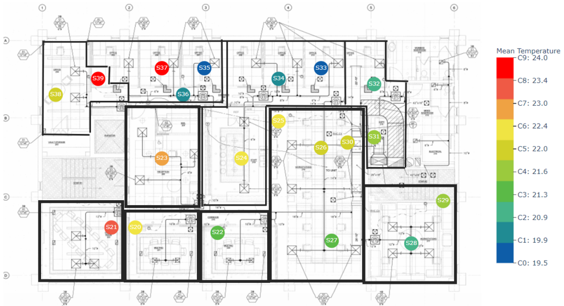
Figure 2.7: K-means cluster results with zones in floor 2. The legend shows the mean temperature values of each cluster
