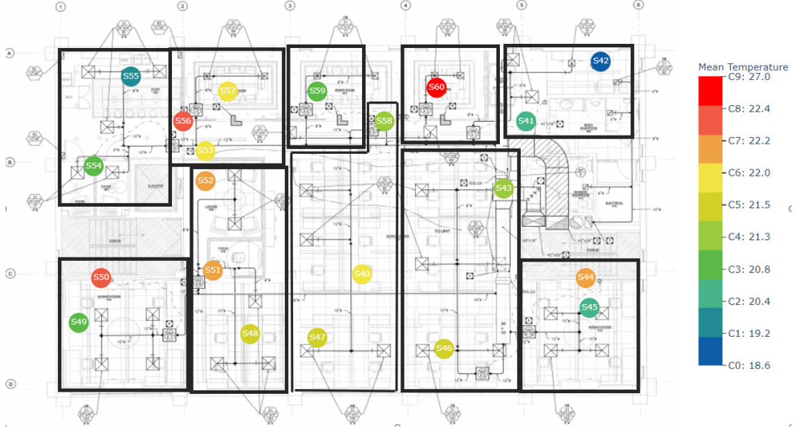
Figure 2.8: K-means cluster results with zones in floor 4. The legend shows the mean temperature values of each cluster
