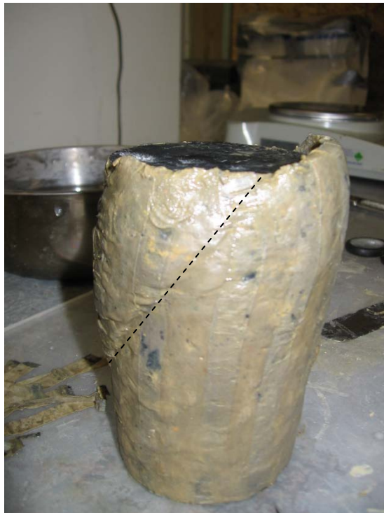
Figure 5.7b – Triaxial Test Failure Surface, Sample T8
