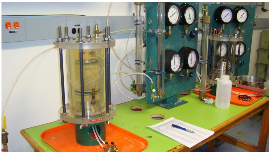
Figure 5.3 – Flexible Wall Permeameter Test Apparatus
