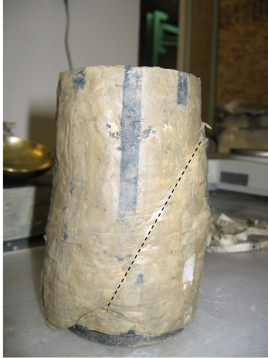
Figure 5.7a – Triaxial Test Failure Surface, Sample T7
