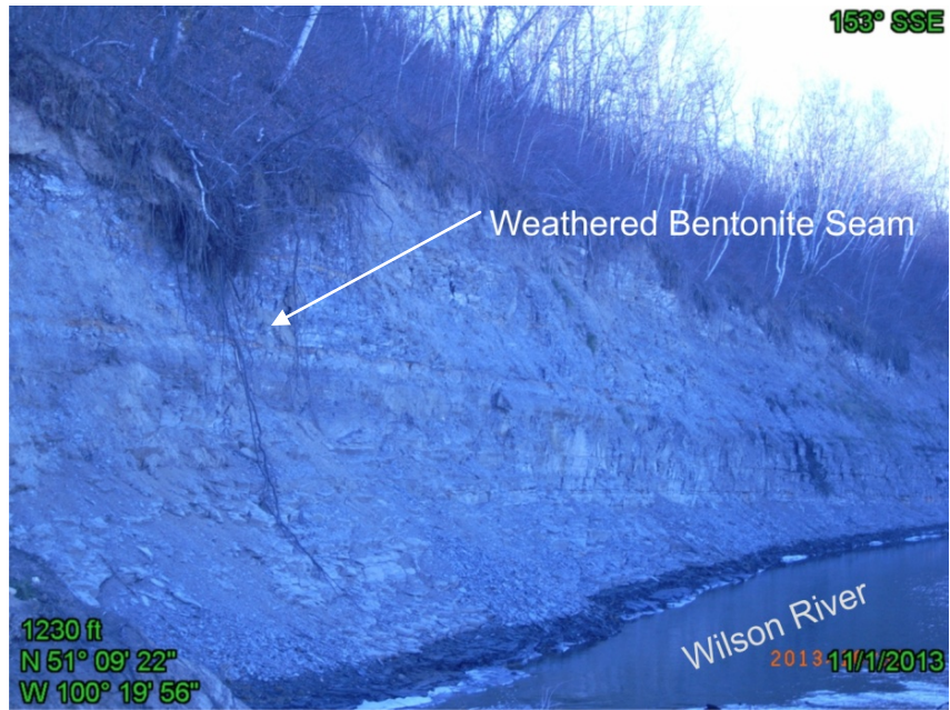
Figure 3.9 – Ashville Formation Outcrop at Wilson River (Note - weathered bentonite seam)
