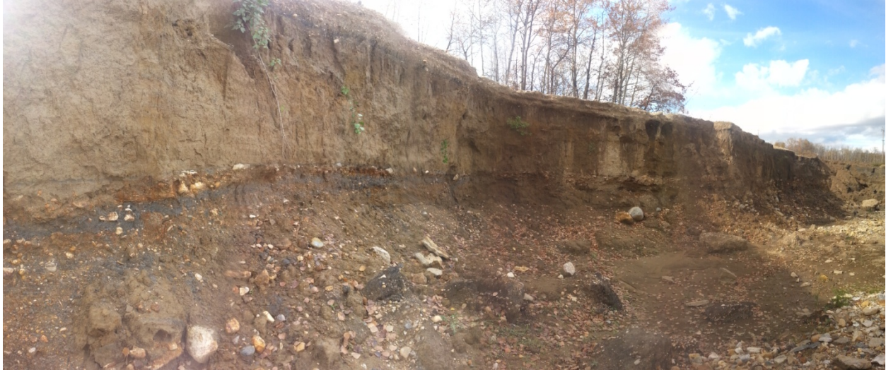
Figure 3.17 – Alluvial Sands and Gravels Beneath Mile Road 121W
