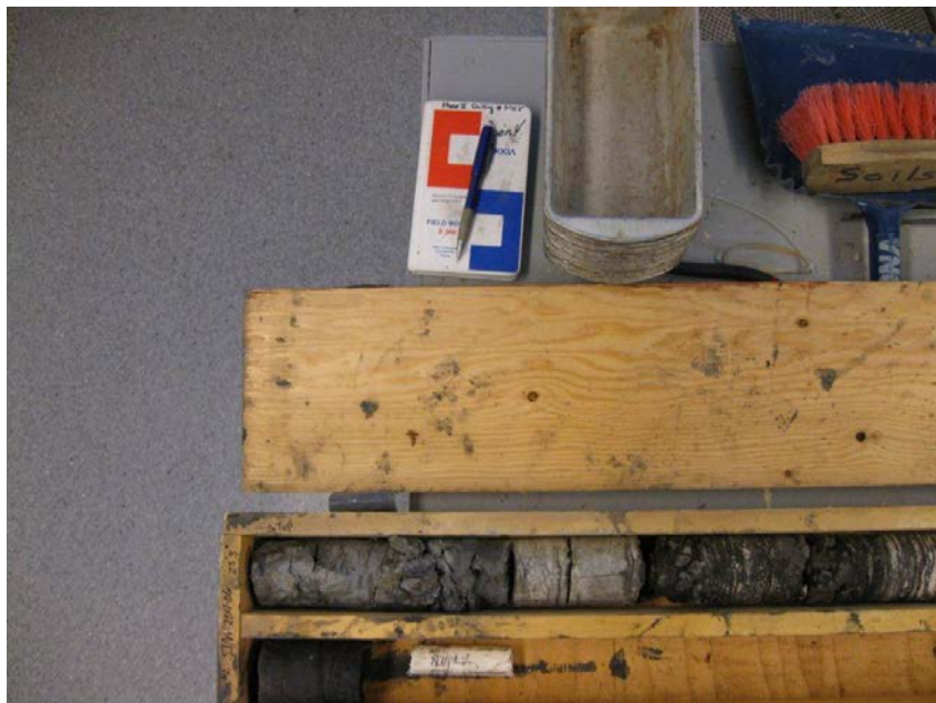
Figure 4.10 – Blue-Grey Bentonite Seam, Sample C16, TH2011-06
