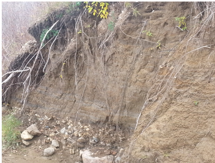
Figure 3.16 – Stratified Alluvial Sediments Beneath Mile Road 121W
