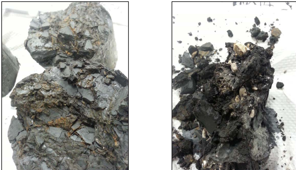
Figure 7.4a (left) – Weathered, Fractured Clay Shale; Figure 7.4b (right) – Gravel Sized Limestone Fragments (TH2011-06, Sample T11)
