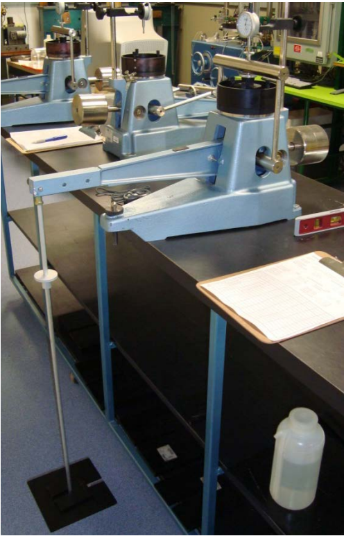
Figure 5.10 – Typical Oedometer Test Apparatus
