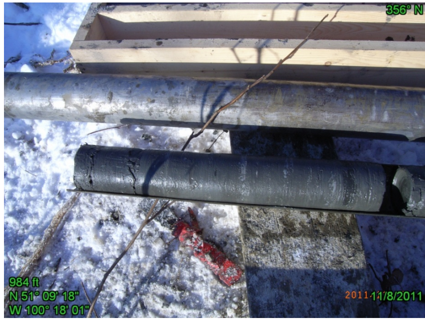
Figure 4.5 – Clay Shale Core Sample During Phase II Drilling
