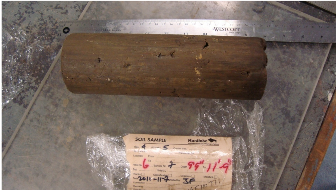
Figure 4.7 – Typical Extruded Shelby Tube Sample (T07, TH2011-06)
