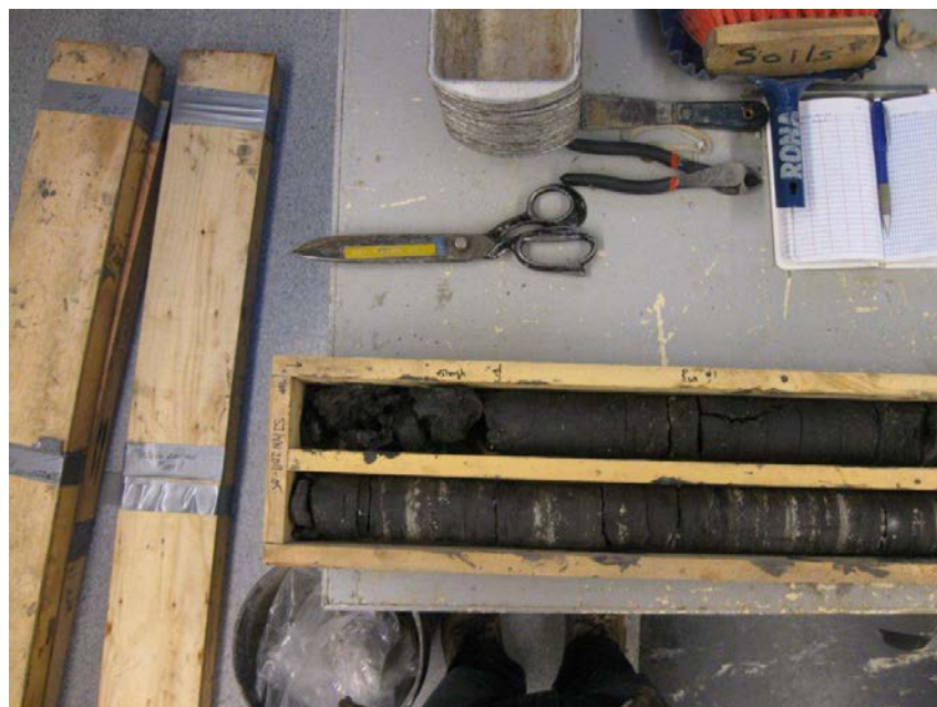
Figure 4.6 – Clay Shale Core Sample (Lower sample shown in Figure 4.5)
