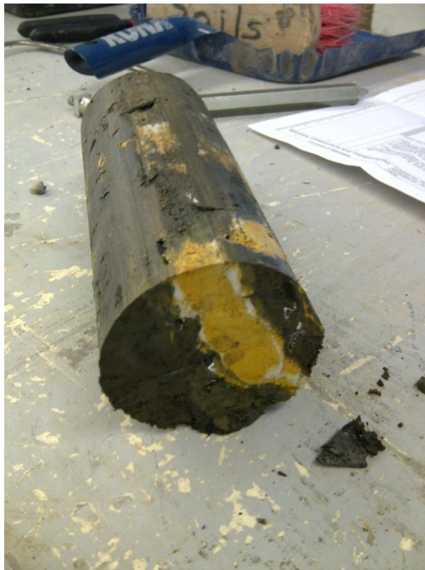
Figure 4.8 – Weathered Bentonite Near Till/Shale Contact (TH2011-06)
