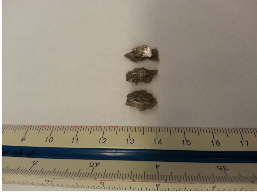
Figure 3.19 – Selenite Crystals Observed in Till-Like Soils
