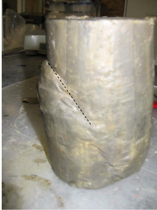
Figure 5.7c – Triaxial Test Failure Surface, Sample T9
