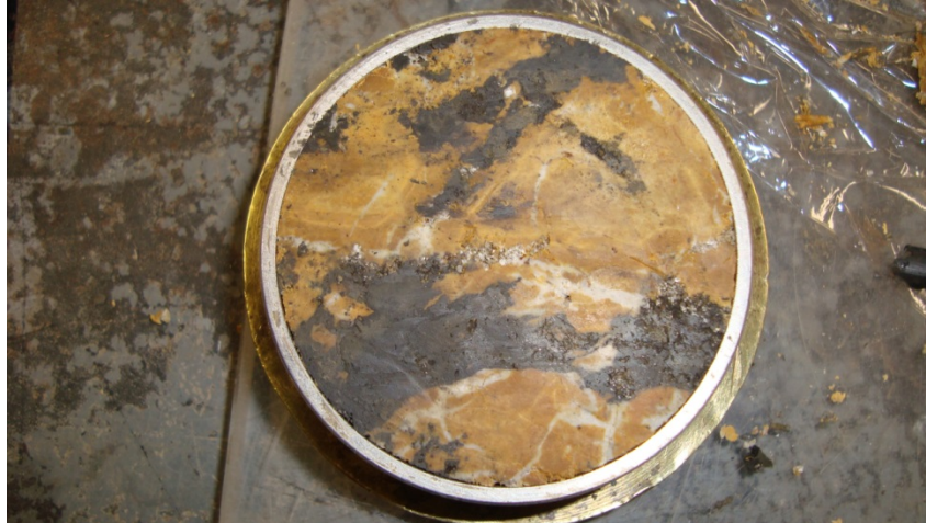
Figure 5.11 – Specimen From Sample T10 in Cutting Ring (Note the yellowish oxidized bentonite)
