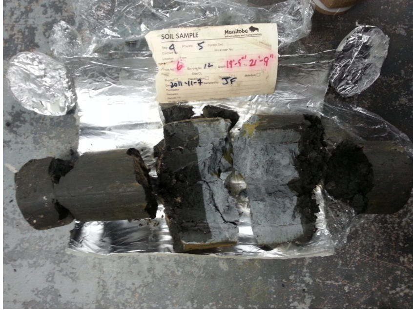
Figure 4.9 – Blue-Grey Bentonite Seam, Sample T12, TH2011-06
