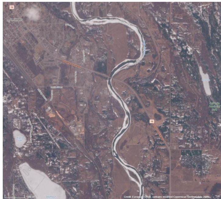
Figure 3.10. Asymmetric partially ice cover in meandering river: (a) Dauphin River, Manitoba, Canada, Dec 2014 (freeze-up season) (Images courtesy of S. Clark and A. Wall); (b) Bulkley river, British Columbia, Apr 2023 (break-up season) (Images courtesy of USGS).
