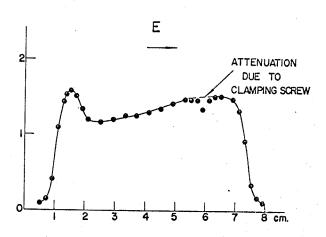
the high power drift. As the drift proceeds reducing the area of the core, the effect becomes more and more pronounced. This non-uniform shape of the core presents no great problem when only direct gamma-ray spectra are to be investigated but it does give rise to serious timing problems when coincidence experiments are performed. The timing characteristics of Ge(Li) detectors will be discussed in Chap IV.
