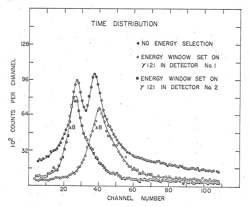
where in the detector the electron-hole pairs have been produced. The solid lines in Fig. 4-12 represent the variation in time required to fire the discriminator versus energy of incident gamma ray. As can be seen from the diagram this variation for detector 1 differs from that of detector 2. This can be caused by having unequal depletion depths or unequal collecting fields or a combination of both.
