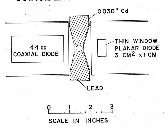
facing the planar detector in order to reduce the number of lead x-rays observed by this diode. Fig. 6-3 shows the "coincidence singles" obtained with this type of geometry.
