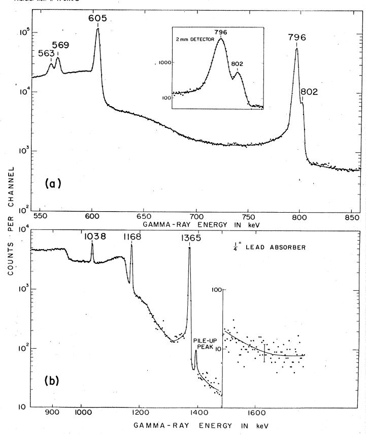
system (Patwardham 1964). The inset shows the 796-802 keV doublet, as recorded by the RCA detector with 2.0 mm depletion depth and  $0.8~{\rm cm}^2$  cross-sectional area.
