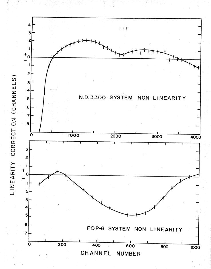
Nuclear Data 3300 system. The A.D.C.'s used with the PDP-8 system preferred unipolar rectangular pulses and these were produced from the Tennelec TC250 biased amplifier. While it was unnecessary to use the biased amplifier with the N.D. 3300 system, it was used for the comparison with the PDP-8 system shown in Fig. 2-6.
