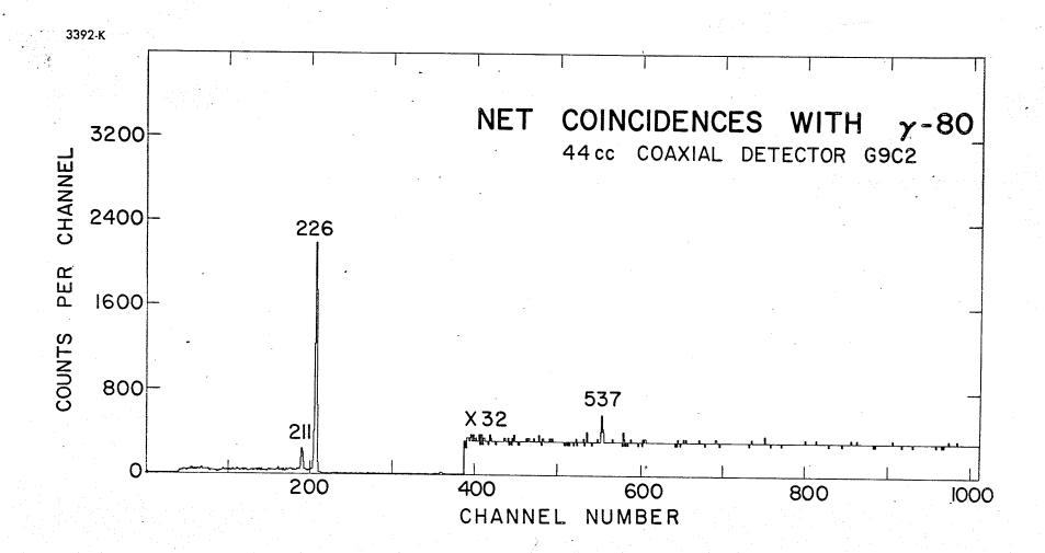
Net coincidence spectrum with  $\delta$ -226. Spectrum shown was recorded by planar detector in coincidence with  $\delta$ -226 in coexial detector.
