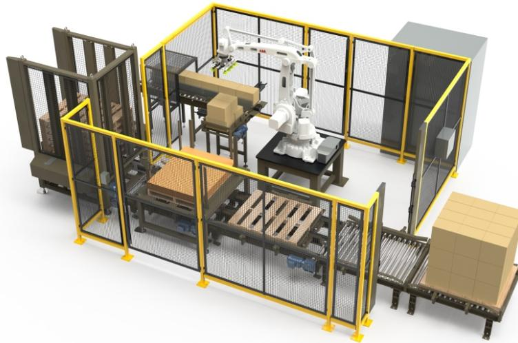
Figure 1.1: An example of a robot cell for palletizing. [1].
