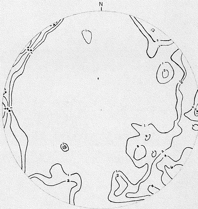
CONTOUR DIAGRAM OF POLES TO 198 MAFIC DYKES CONTOUR INTERVAL IN % 4
