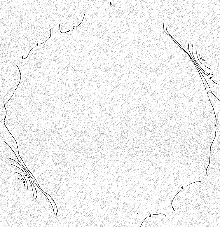
CONTOUR DIAGRAM OF POLES TO 301 JOINTS GRID = ONE PER SQUARE MILE CONTOUR INTERVAL IN % = 8
