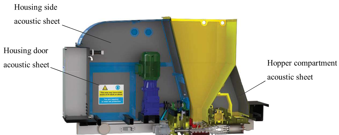
Figure 35: Acoustic dampening material sheets applied to the housing and hopper compartments
