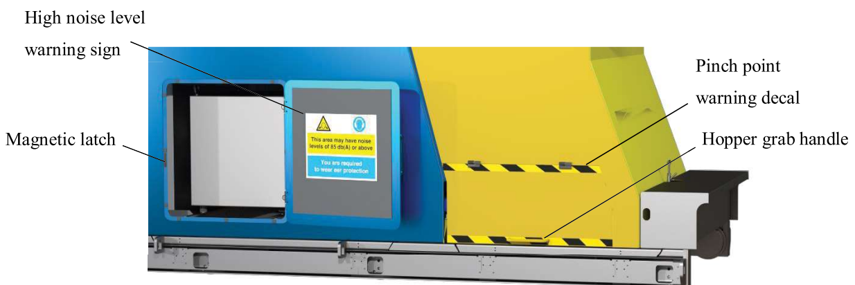
Figure 10: Redesigned hopper and housing extruder doors with safety warning signs
