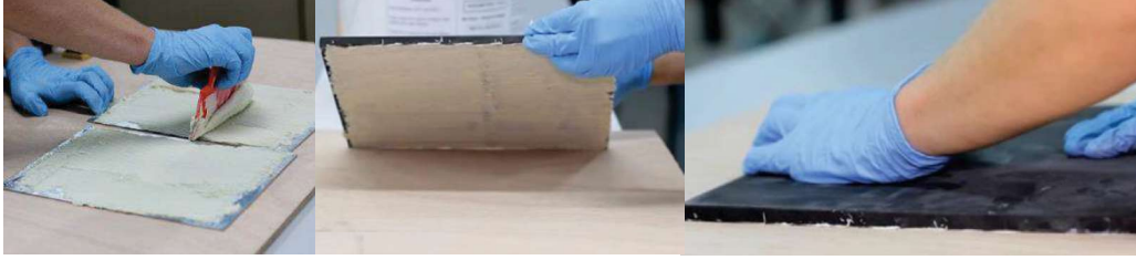
Figure 45: Pyrotek DC30 polyurethane adhesive applied to a Decidamp tile [16]
