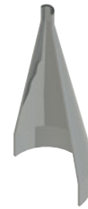
Figure A - 3: Expansion tube where the cross section area of flow expands
