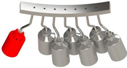
Figure 1: Approximation of the Current Oil Collection System
