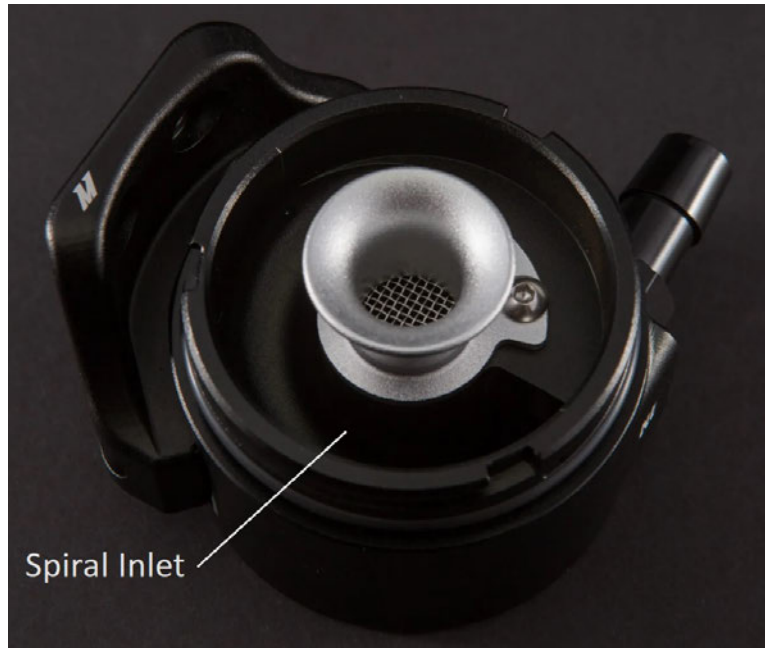
Figure 6: Spiral inlet of the catch can lid [9]
