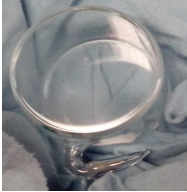
Figure 3.9: Paraffin coated Rb cell. The cell contains natural rubidium with stable isotopes ^{85}\text{Rb} and ^{87}\text{Rb} . The cell is cylindrical, 5 cm long and 5 cm in diameter with optical flats on the ends.
