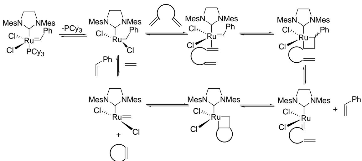
**Scheme 3.5.10:** Catalytic process in ring closing metathesis reaction.<sup>123</sup>
