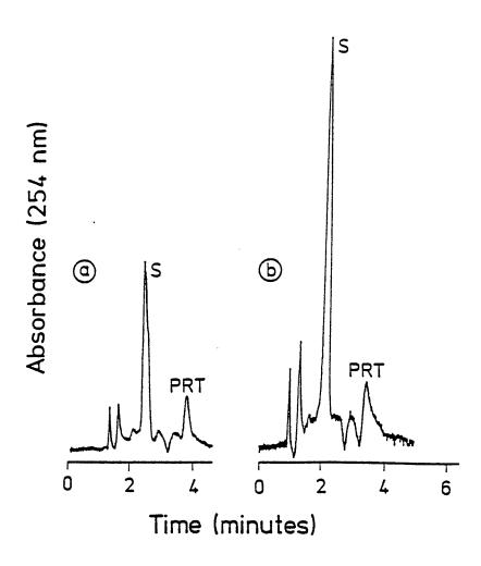
Figure 3.3 Chromatograms of crude PRT extracts obtained from two separate fermentation batches of *Penicillium roqueforti*, 100 ml of YES culture medium. Eluent: methanol-water (65:35, v/v); flow rate, 1.0 ml/min; peak S=methanol.
