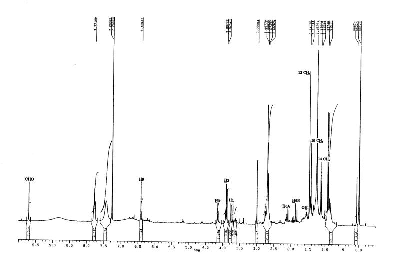
Figure 4.12 The 300 MHz <sup>1</sup>H NMR spectrum of the succinylation product (in CDCl<sub>3</sub>) of 5.0 mg of PR alcohol using procedure 4 (TMS as internal standard).
