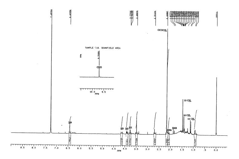
Figure 4.11 The 300 MHz <sup>1</sup>H NMR spectrum of the succinylation product (in CDCl<sub>3</sub>) of 1.0 mg of PR alcohol using procedure 4 (TMS as internal standard).
