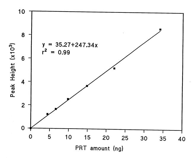
APPENDIX IV - Correlation of PR imine amount and HPLC peak height. Eluent: acetonitrile-water (60:40,  $\rm v/v$ ).
