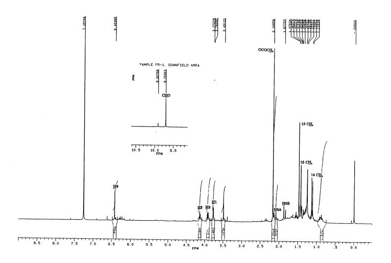
Figure 4.10 The 300 MHz <sup>1</sup>H NMR spectrum of the succinylation product (in CDCl<sub>3</sub>) of 1.0 mg of PR alcohol using procedure 3 at room temperature (TMS as internal standard).
