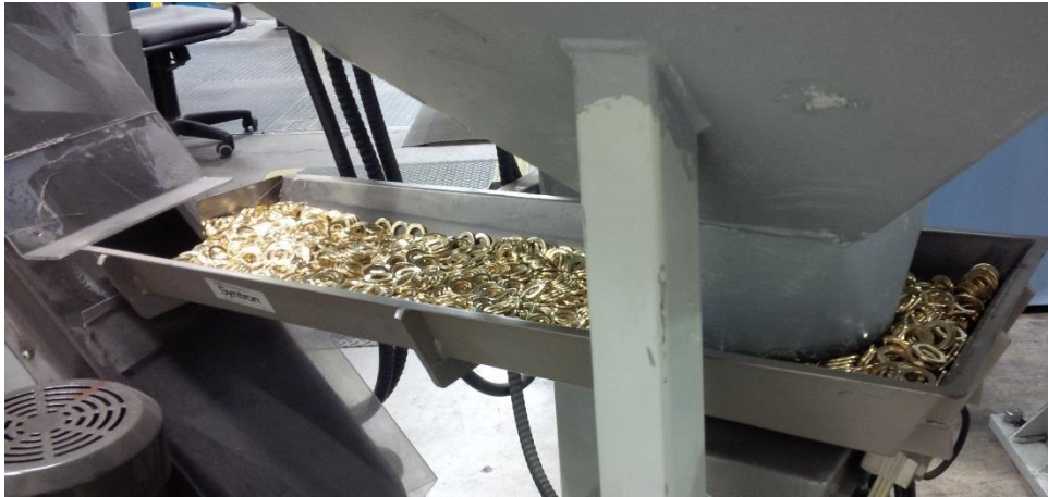
Figure 45. VFP from F-line conveyance system on F3 press [6].
