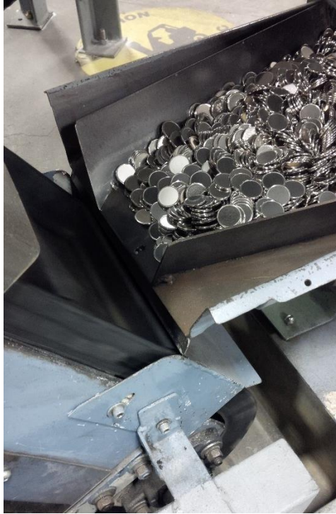
Figure 6. VFP to belt transfer point [7].
