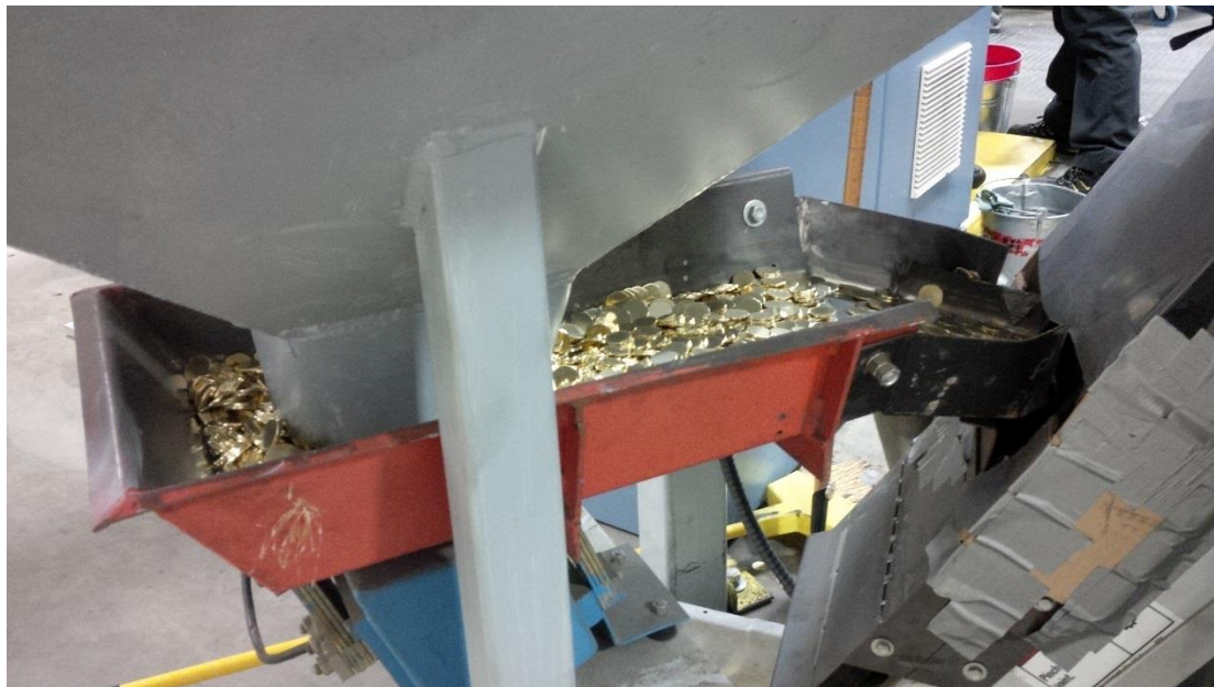
Figure 44. VFP from F-line conveyance system on F5 press [6].
