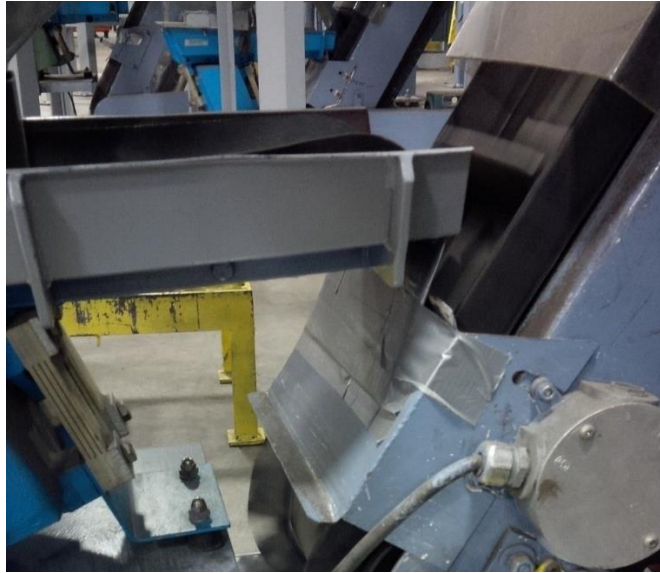
Figure 7. Metal fender at the outfeed of the VFP [7].
