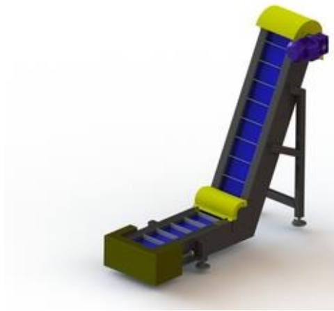
Figure 8. Inclined conveyor designed by Barlow Manufacturing [8].
