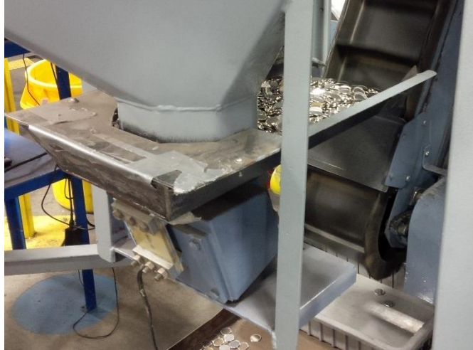
Figure 4. VFPR temporary cover and conveyance system [7].
