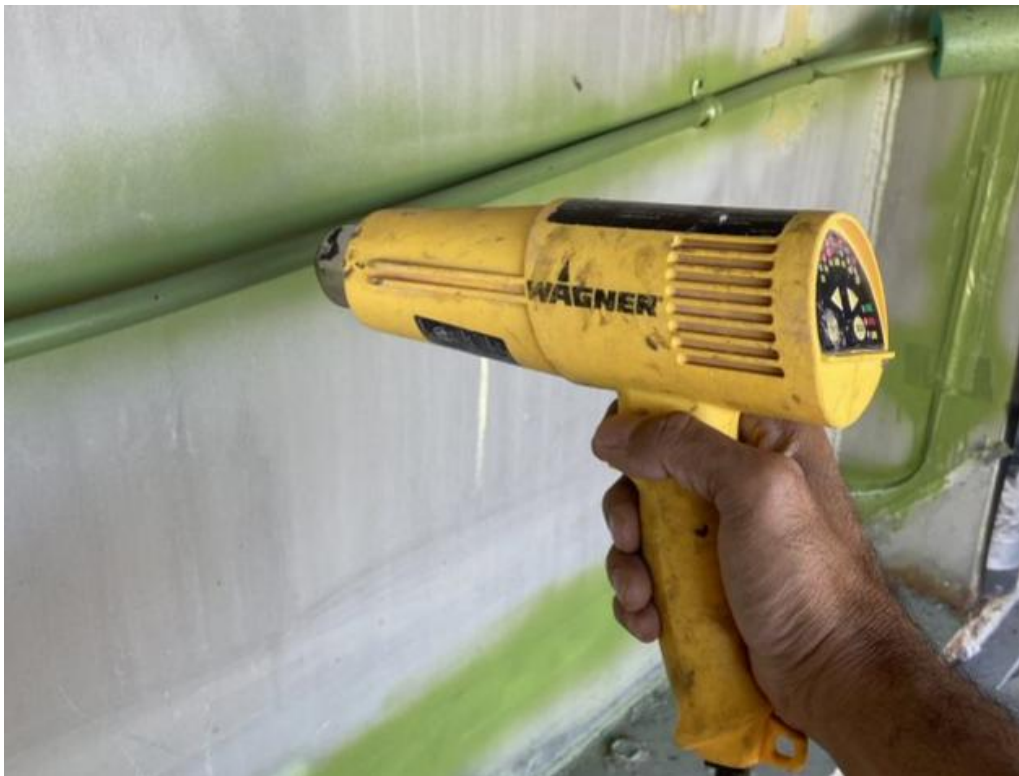
Figure 7.7: Thermal localization of start and end points of each FOS sensor loop
