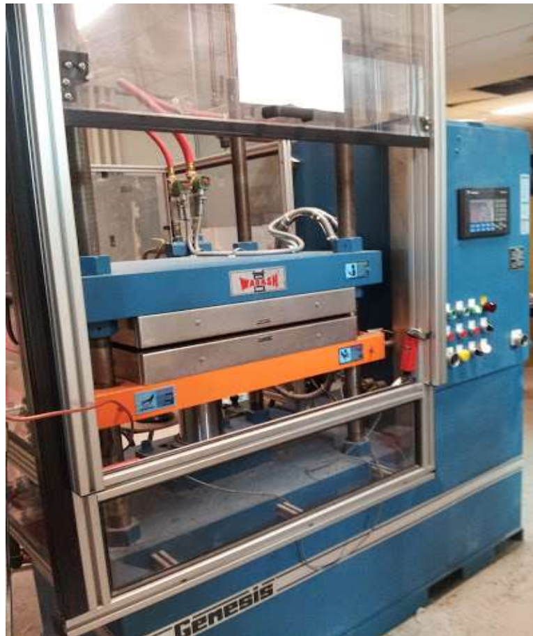
Figure 4.1: Carver hydraulic hot press used in manufacturing of hybrid composite panels
