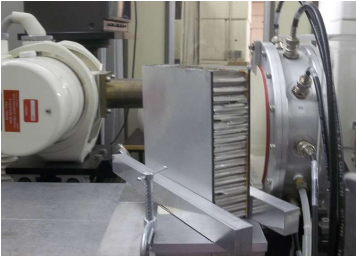
Figure 5.9: Set-up of DSP panel at 30^\circ angle to the beam direction
