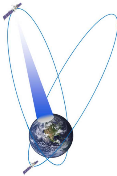
Figure 1.1: Two satellite constellation for continuous coverage of Canadian Arctic region
