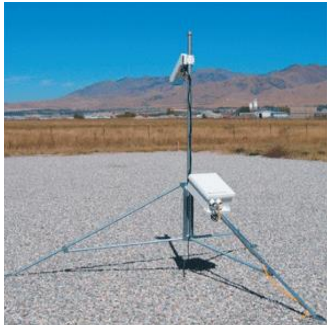
Figure 4.6 CS110 electric field sensor and its installation, manufactured by Campbell Scientific.
