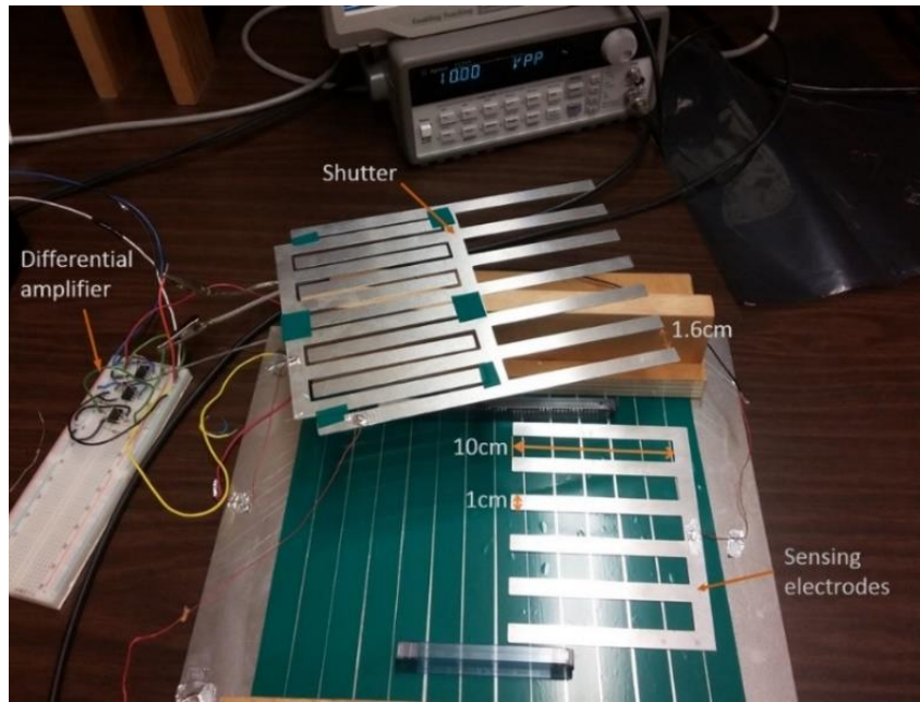
Figure 8.6 Shutter, sensing electrodes and amplifier.
