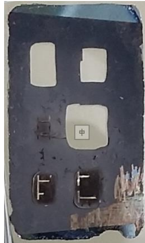
Figure 5.12 Plasma photoresist clean use high RIE power.
