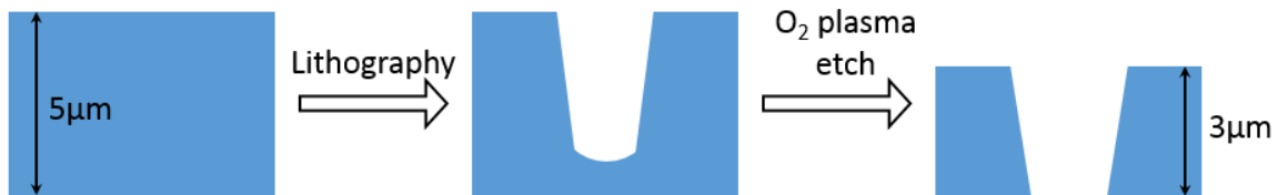
Figure 8.31 SU-8 finger and shutter release.
