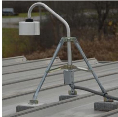
Figure 4.5 EFM-100 Electric Field Monitor and its installation, manufactured by Boltek.
