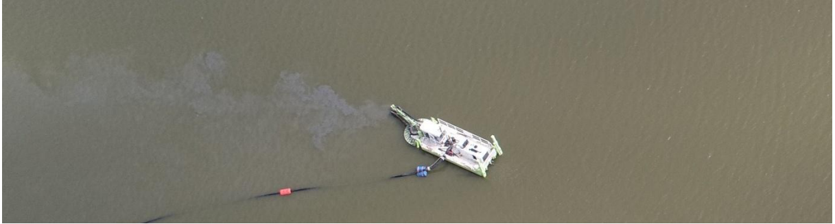
Figure 5-6 Sediment plume downstream of an Amphibex unit during dredge operations
