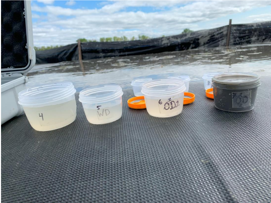
Figure 5-2 Representative turbidity samples collected inside and outside the containment barrier
