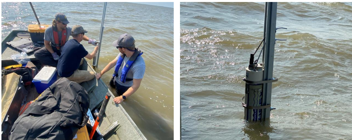
Figure 5-8 Hydrolab ® installation in Netley Lake
