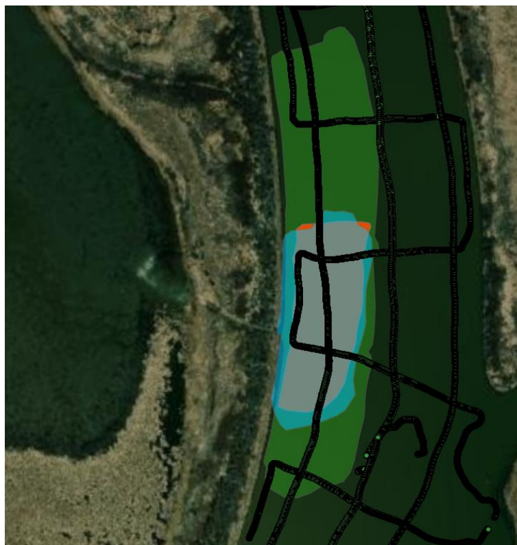
Figure 3-29 Sounding path of the bathymetric survey conducted by Manitoba Hydro in 2018
