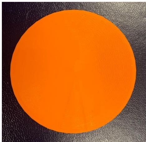
Figure 3.4: 3D printed PLA disc sample using infill setting as concentric by Cartesio v12 W printer
