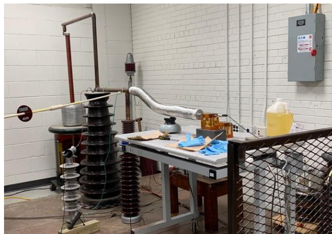
Figure 3.18: Experiment setup for partial discharge measurements in laboratory
