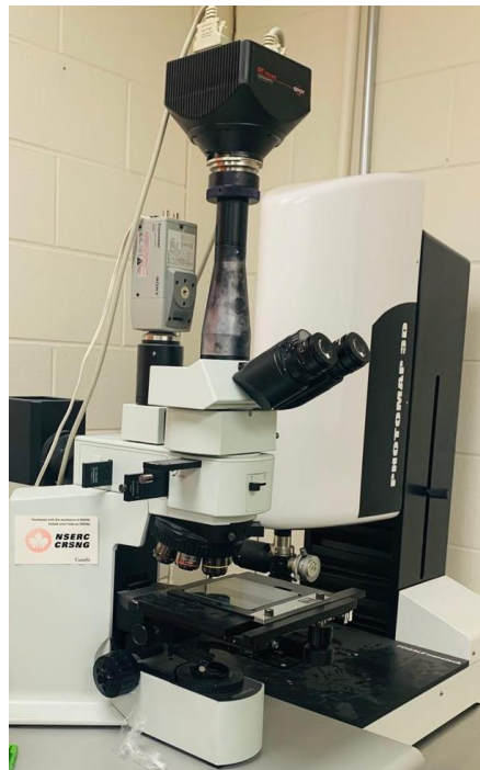
Figure 3.8: Olympus BX511TRF optical microscope used to study the sample surface.
