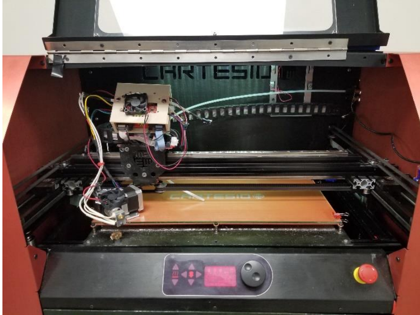
Figure 3.2: Image of the Cartesio v12 W 3D Printer manufactured by MAUK Custom Creations with multiple components including extruder, a nozzle head, heated printer bed and connections with computer and power.
