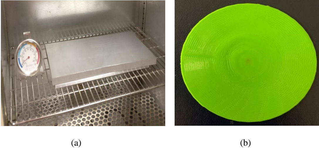
Figure 3.5: (a) Heat treatment setup for compressing PLA discs between two aluminium plates at 90 °C in an oven. (b) Visible warps formed in the sample after heat treatment in the oven.
