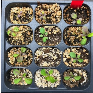
Figure C2. Germination trial results. From left to right: mix 1 (35% MD1, 35% Peat, 30% Perlite), mix 2 (70% MD1, 30% Peat), and mix 3 (100% MD1).
