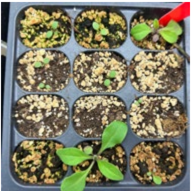
Figure C3. Germination trial results. From left to right: mix 4 (35% MD 2, 35% Peat, 30% Perlite), mix 5 (70% MD2, 30% Peat), and mix 6 (100% Media Design 2).
