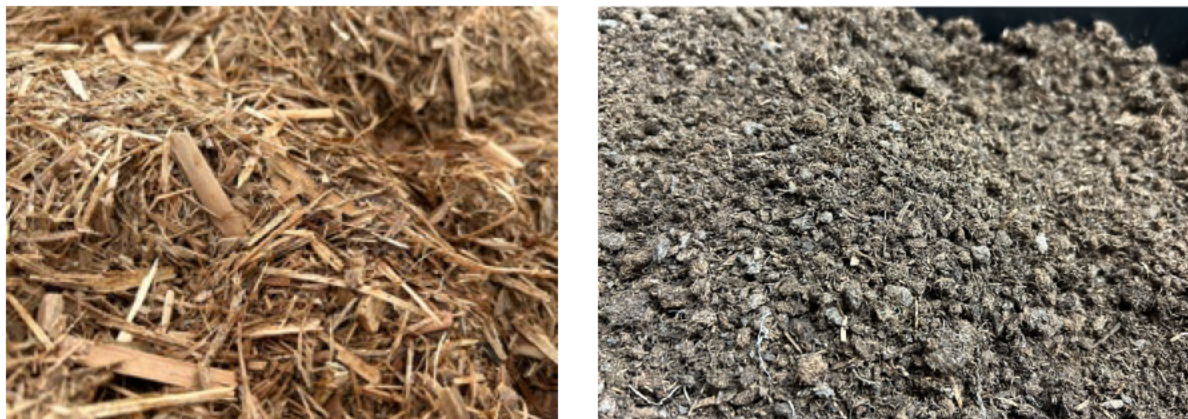
Figure 7. Non-composted Typha (left) is coarser in texture, meaning it contains larger particles, and lighter in colour compared to composted Typha (right)
