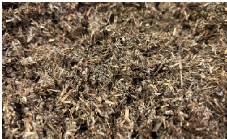
Figure 8. Non-composted, milled Typha is lighter in colour than composted Typha and finer in texture than Raw Typha (shown in Figure 7)
