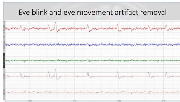
*Figure 3-2. EOG correction of EEG data recorded during the SST. (Top to bottom) F8 before correction; F8 after vEOG correction; F8 after vEOG and hEOG correction; vEOG; hEOG.*
