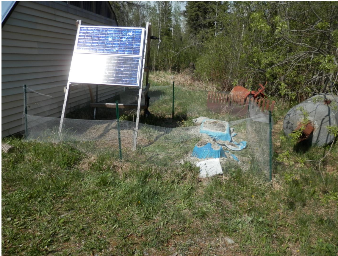
Figure 5.2: A typical Canadian SPREE station with its seismometer and electronic box buried underground.
