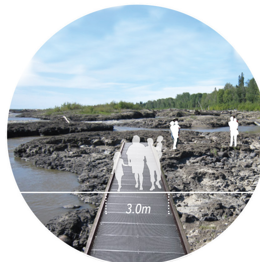
Developed Trail - Metal Grate Walkway
