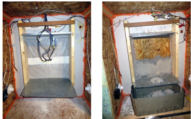
Figure 3-15: Cellulose density test setup
