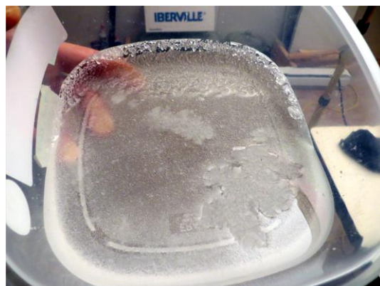
Figure 3-9: Crystal formation of Potassium carbonate solution in chamber 3 of fiberglass bldg.
