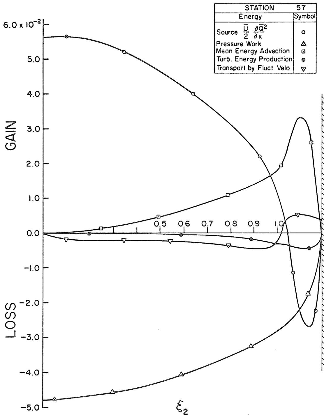
Figure 8: Mean kinetic energy balance at station 57
