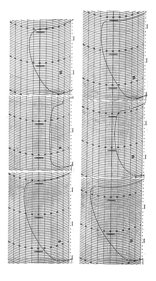
Figure 6c. Extensigrams (at 135 min) of the Seven 1BL/1RS Cultivars at Glenlea 1989. 1, BR 23; 2, 8416-Q06A; 3, 8416-Q06E; 4, 8416-BZ10A; 5, 8416-BZ10C; 6, 8417-BJ03A; 7, 8417-BJ03D.
