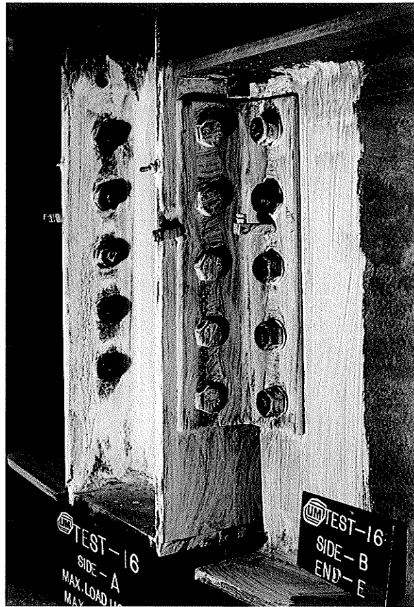
Figure 5.27: Yielding Along the Bolt Lines of the Column Leg of the Angle in the Tension Region of Specimen 16.
