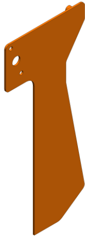
Figure 26: New Side Plate Shape.
