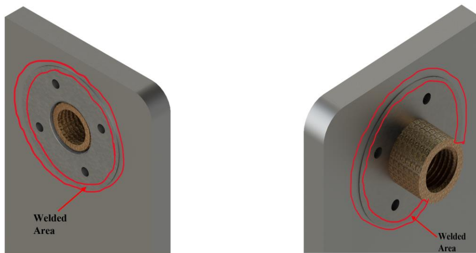
Figure 61: Welded on The Inside (Left) And Outside (Right).
