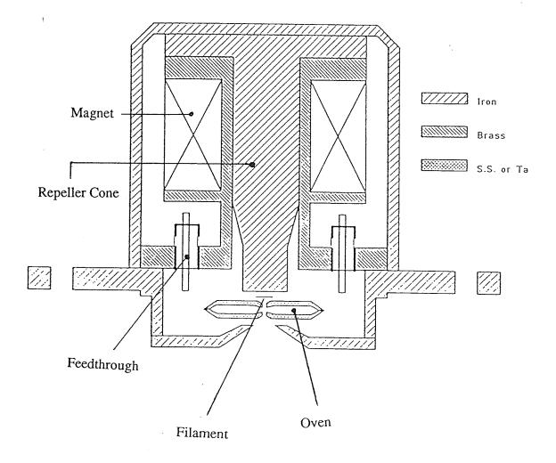
Figure 3.3 Duoplasmatron Ion Source
