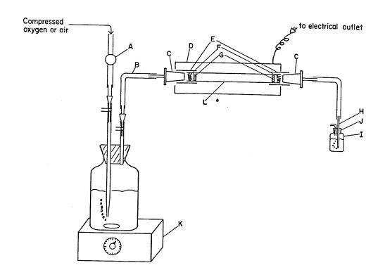
A. Gas metering valve (if required); B. flexible hose; C. plastic adapter (or attach hose directly to tube); D. Tube furnace; E. silicone hose (unless vycor tubes extend from furnace); F. steel wool; G. quartz wool; H. disposable glass pipette; I. 20 mL glass scint. vial with CO<sub>2</sub> trap; J. silicone stopper (use on original sample bottle, optional on scint. vial); K. magnetic stir plate; L. Vycor tubing packed with copper oxide.
