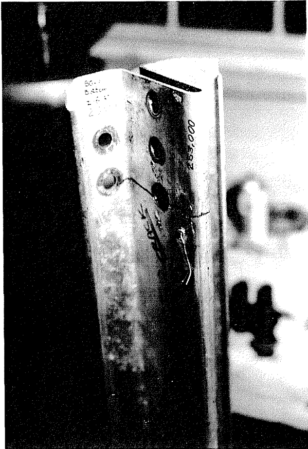
Figure 4.90 : Failure of T-shaped Section (BG).
