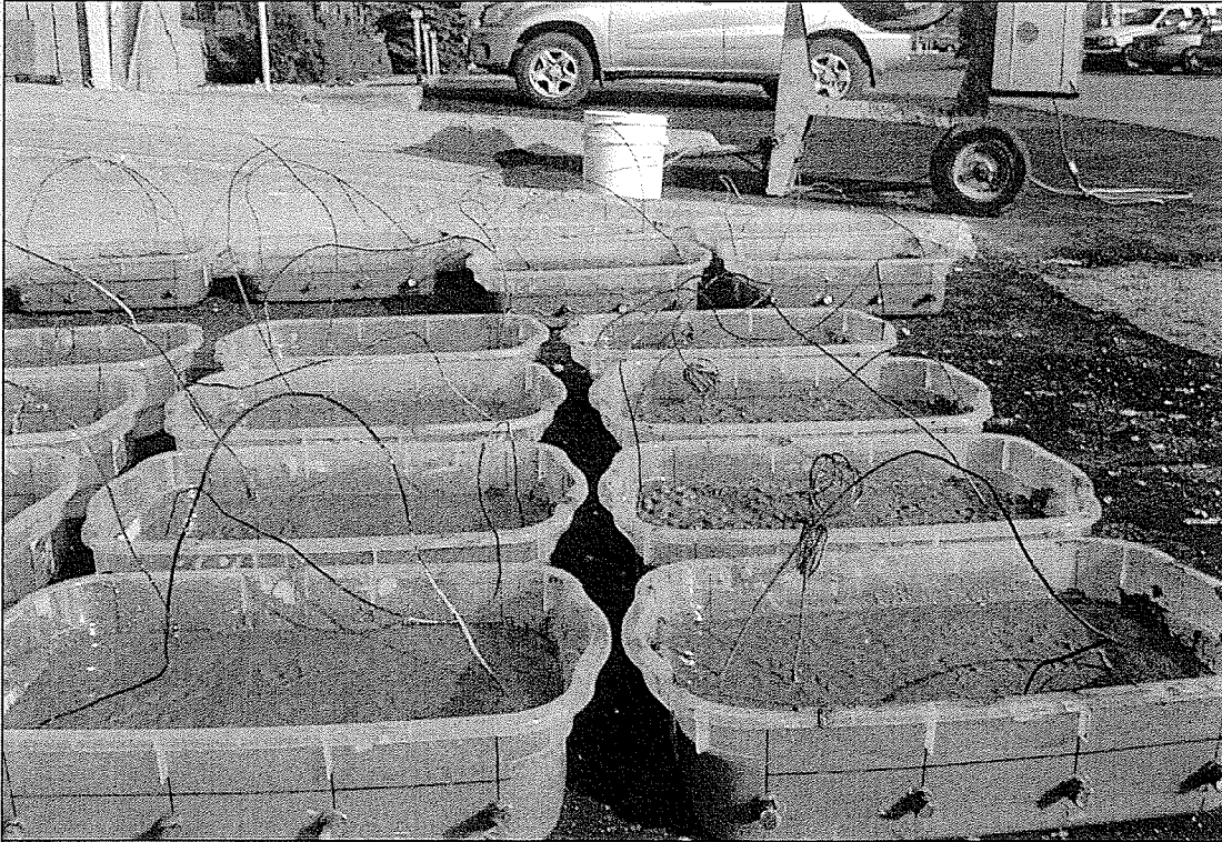
Figure 3-3: Photo of concrete slab specimens on day of casting
