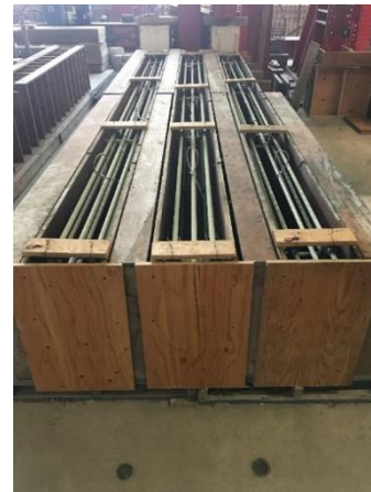
b) Continuous beams
