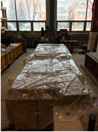
c) Beams in curing
