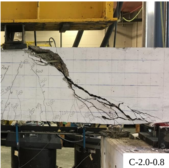
Figure 4.2: Modes of failure of test beams.
