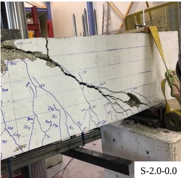
Figure 4.2: Modes of failure of test beams.
