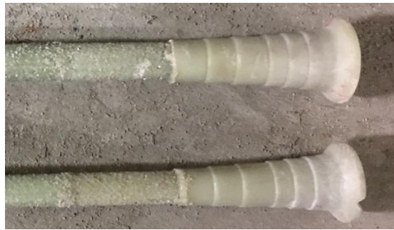
Figure 3.4: Photos of the used headed GFRP bars
