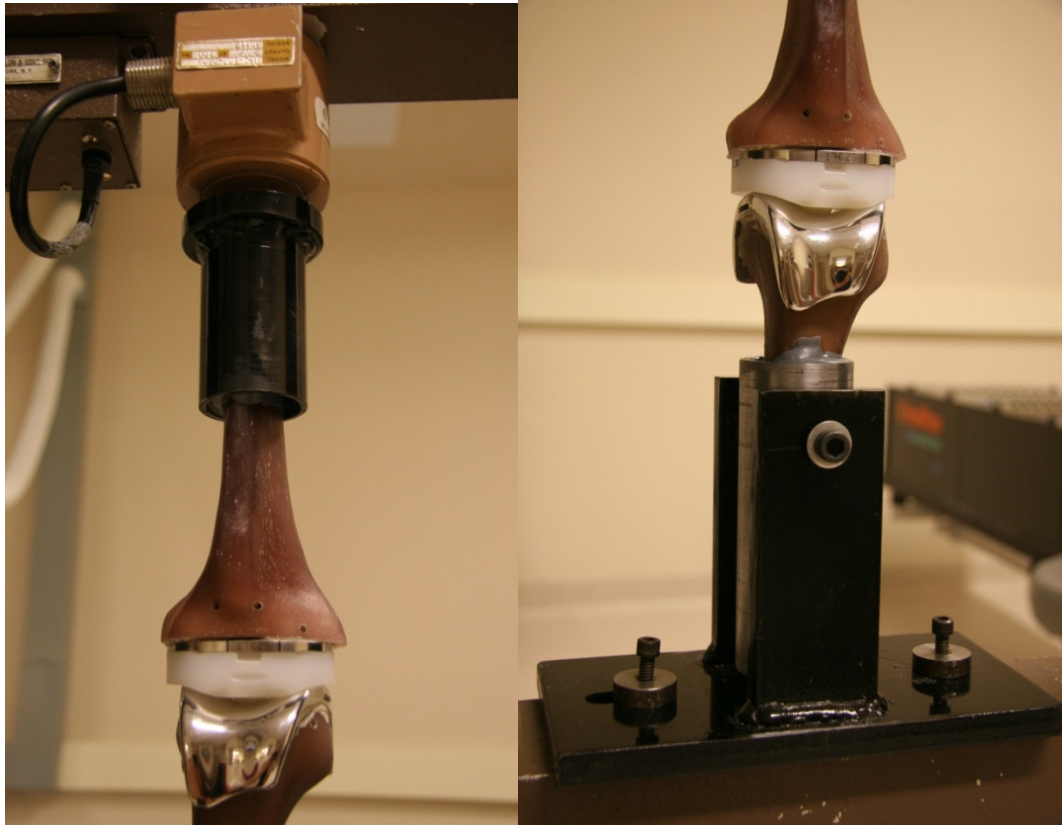
Figure 30: A) Tibia bone mount fixed to the load cell which is fixed to the frame, B) Femur bone mount fixed to the lower cross bar of the load frame.
