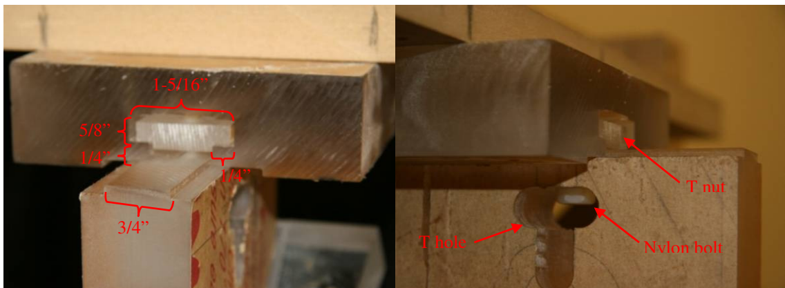
Figure 24: A) T-groove and corresponding “shoulders” dimensions. B) T-shaped hole in flexion block, nylon tightening bolt, t-nut.
