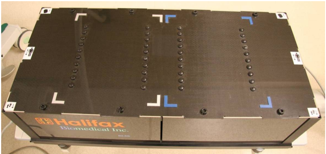
Figure 7: Halifax Biomedical uniplanar calibration cage showing the control markers on either side of the cage. The fiducial markers are not visible as they are located inside this enclosed cage.
