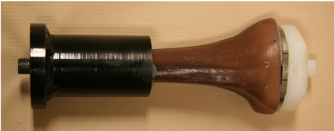
Figure 28: Tibia bone mount with the proximal section of the Sawbones tibia inserted.
