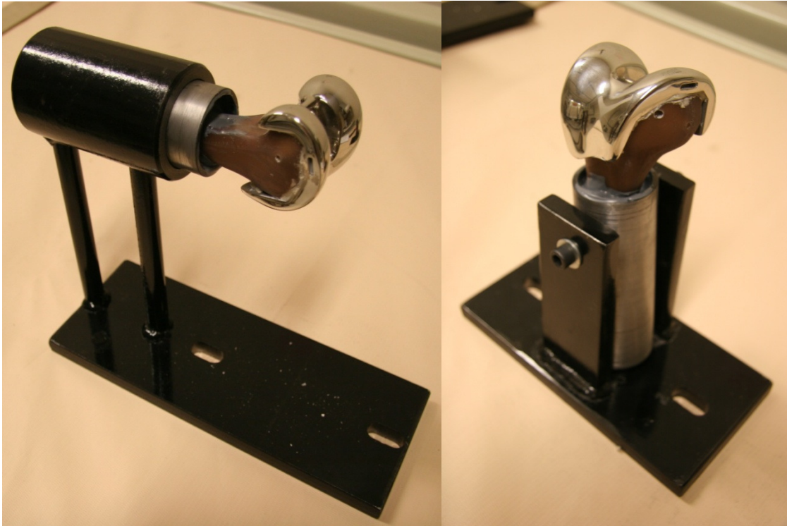
Figure 29: A) Sitting (90° flexed) femur bone mount with dimensions, B) Standing femur bone mount with dimensions.
