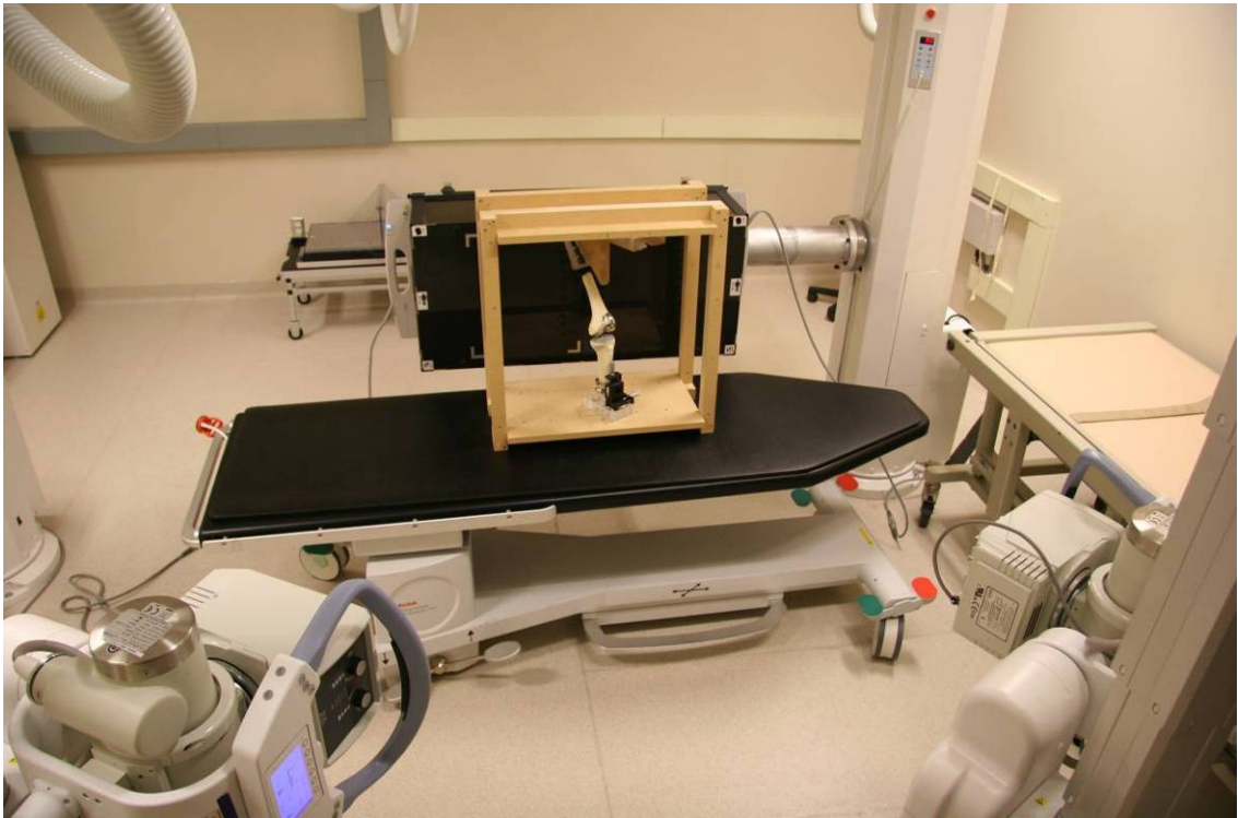
Figure 31: RSA setup with HBI calibration box, DR imaging plates, precision phantom model on wheeled support, and dual x-ray tubes positioned horizontally at 30^\circ to the perpendicular of the calibration box.
