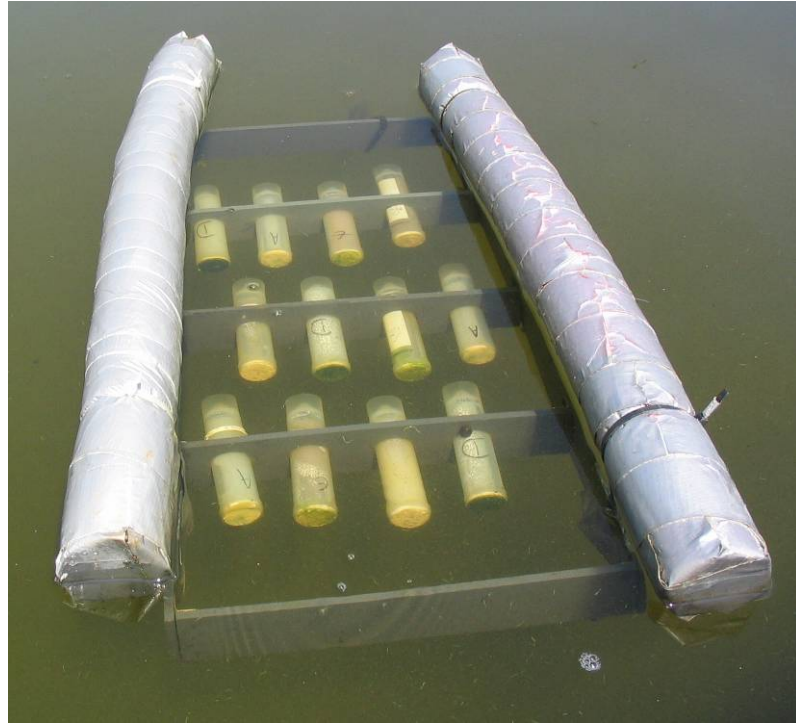
Figure 4-1. Nutrient diffusing substrata frame in farm pond (deployment of nutrient treatments in the frame was random).
