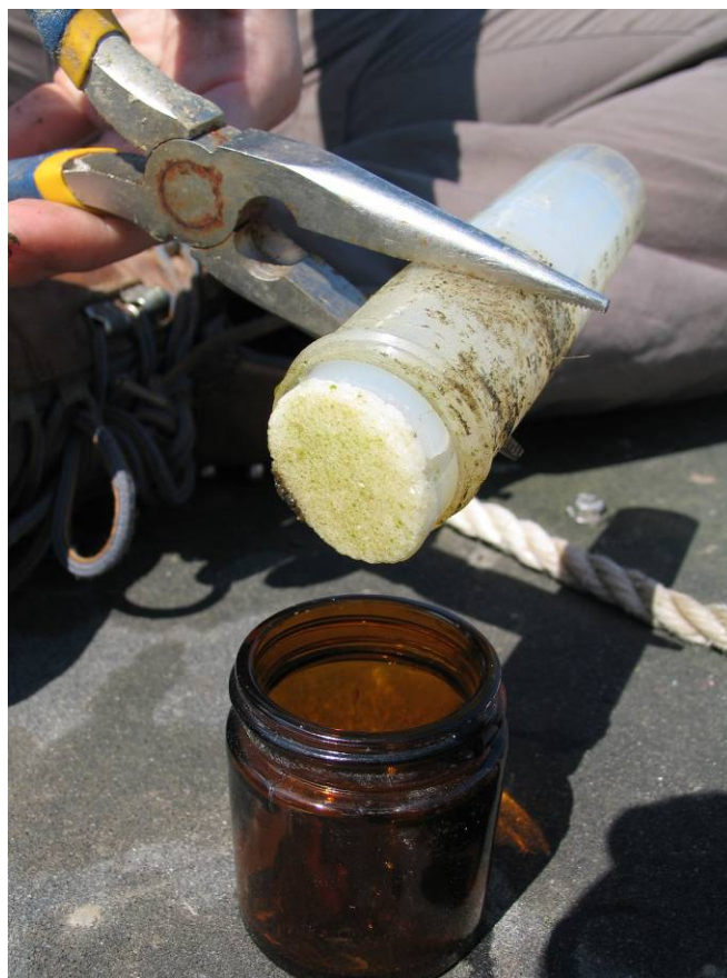
Figure 4-3. Treatment tube being squeezed by pliers to remove silica frit for storage in the brown glass jar.
