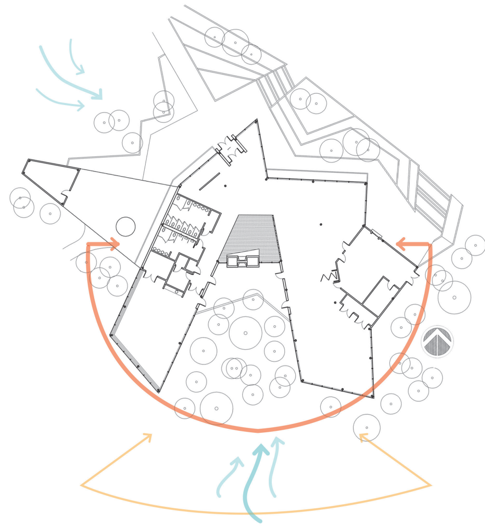
Figure 16. Qualico Family Centre is designed to prevent solar heat gain in summer and maximize heat gain in winter.
