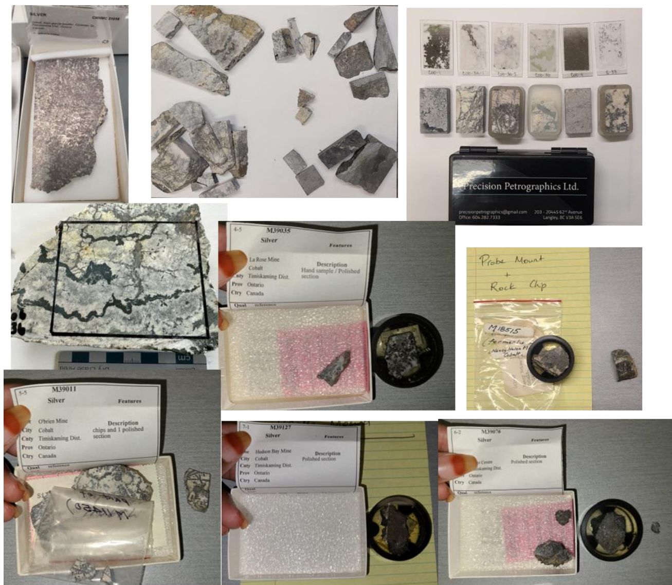
Figure S5. Photos of rock samples, thin sections and pucks of the selected samples from the Cobalt Embayment.
