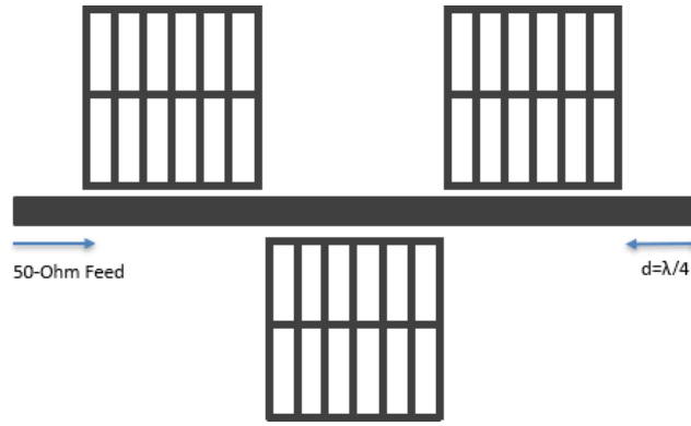
Fig. 2.5: Bandwidth enhancement of TMPAs using three proximity-fed meshed patches [42].
