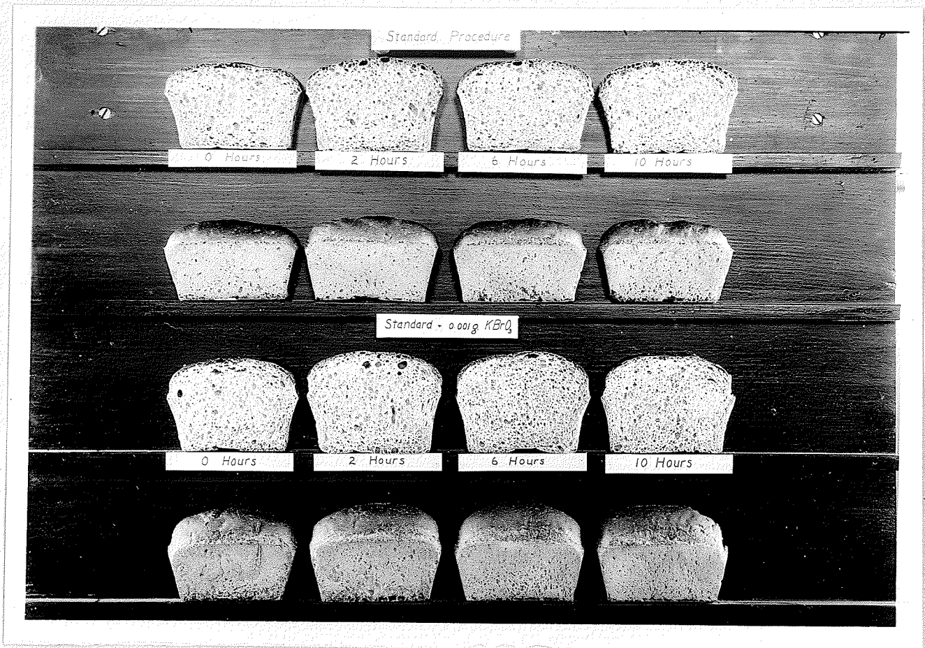
Fig. 9 The Effect of Different Times of Treatment on Low Moisture Germ at 170°C, loaves baked by the Standard and Bromate Procedures.
