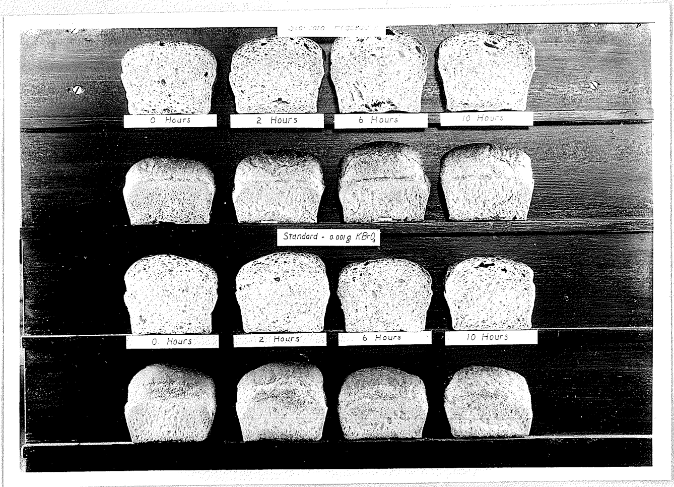
Fig. 13 The Effect of Different Times of Treatment on High Moisture Germ at 170°F, loaves baked by the Standard and Bromate Procedures.
