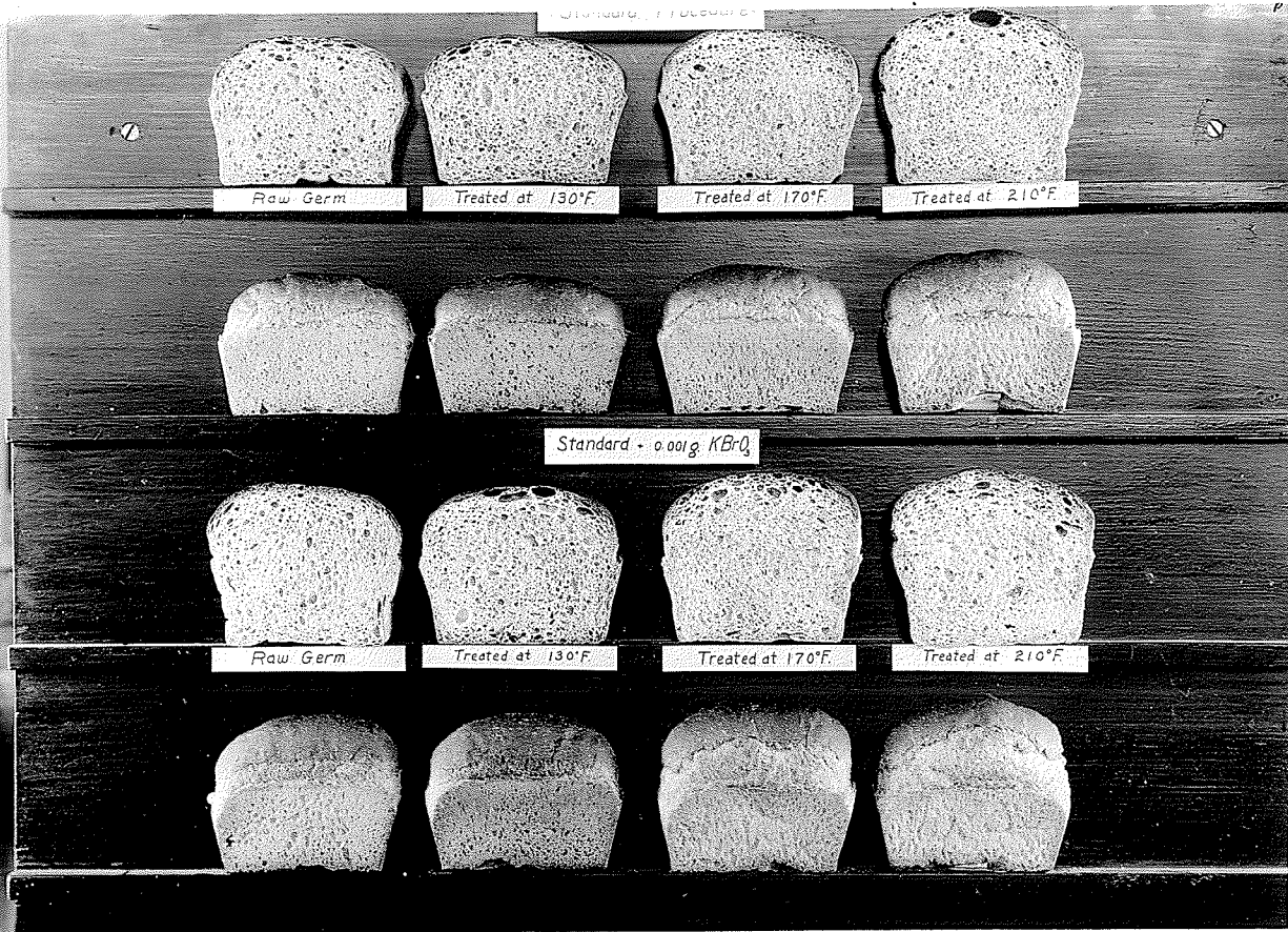
Fig. 5 The Effect of Different Temperature Treatments on Natural Moisture Germ for 3 hours, loaves baked by the Standard and Bromate Procedures.
