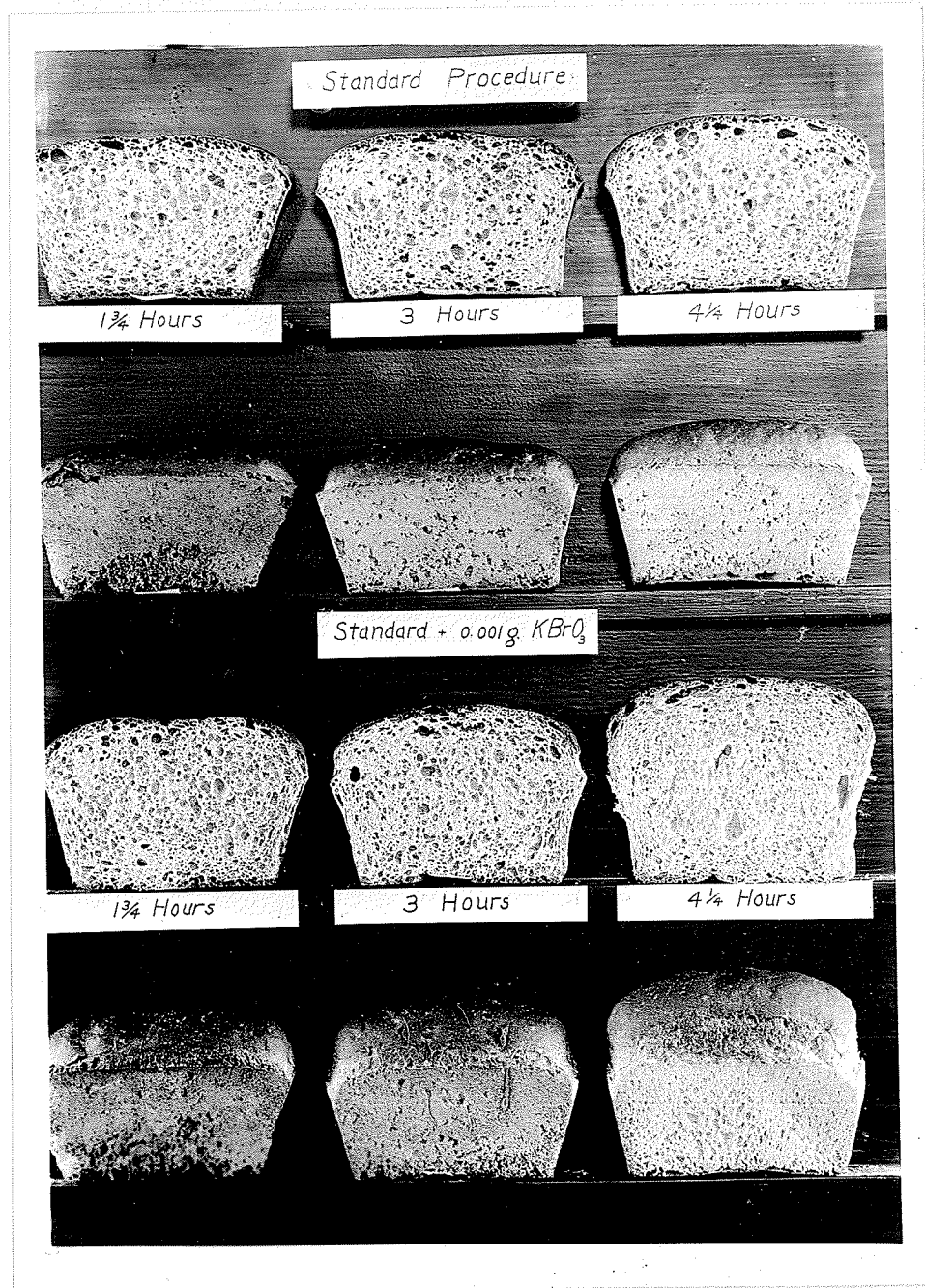
Fig. 17 The Effect of Varying the Fermentation Time on High Moisture Raw Germ, using the Standard and Bromate Procedures.
