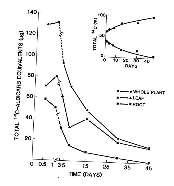
at 12 hours (Table 33). The percent remaining declined rapidly over the 45 day duration of the experiment. At 45 days only 12.1% of uptake was recovered. Conversely 87.9% of  $^{14}$ C activity was eliminated from the plant in 45 days. The rate constant for loss of aldicarb equivalents from the whole plant was found to be 0.05 day<sup>-1</sup>. Subsequently the half-life of aldicarb and equivalents following a single dose root feeding as described, was calculated at 13.9 days.
