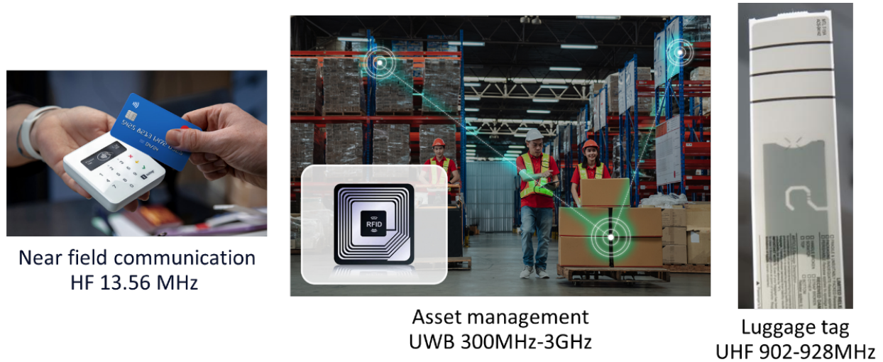
Fig. 2.4: Some examples of RFID applications that operate in different frequency bands in our daily life.
