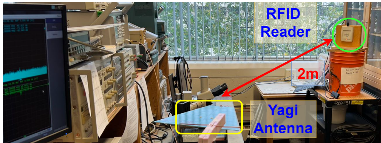
Fig. 5.2: Experiment setup for measuring the RF output of a RFID reader.
