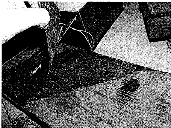
Figure 4.1: Debonded GFRP Sheet
